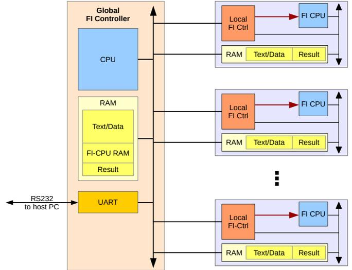
Fig. 1. Architecture of FPGA-based FI system: Multiple Cortex-M0 cores run FI experiments in parallel, while a global FI controller oversees the campaign, resets FI CPUs and memories, configures local FI controllers with concrete fault coordinates, and collects result data.
