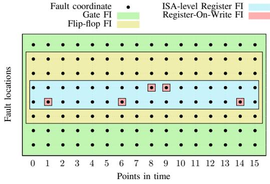
Fig. 2. Overlapping fault spaces for different FI techniques and fault models: Gate-level FI injects into the set of all available CPU gates – i.e. all possible injection (time/space) coordinates, – while the other techniques inject in decreasing subsets thereof.
