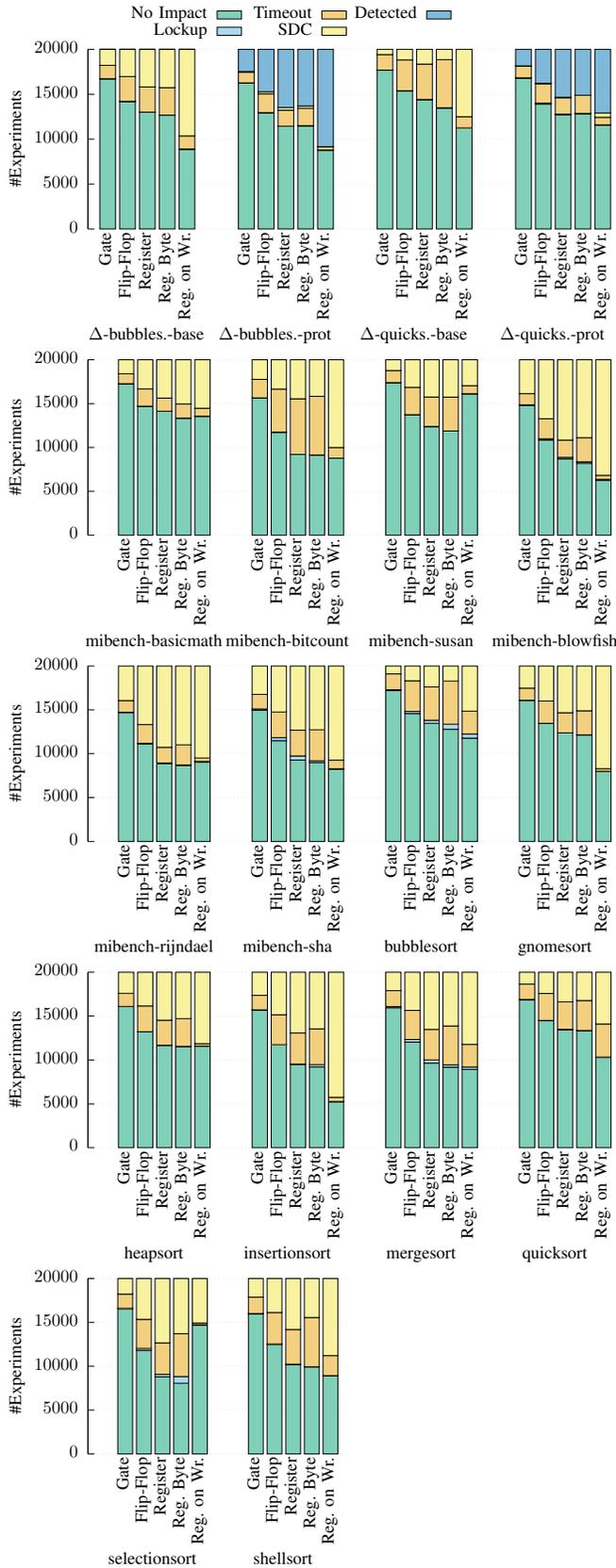
Fig. 3. Raw FI results: Across different FI techniques, for some benchmarks the proportion of specific result types is off by up to an order of magnitude compared to the gate-level baseline.
