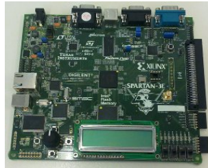
Abbildung 4.6: FPGA Spartan-3E S500
